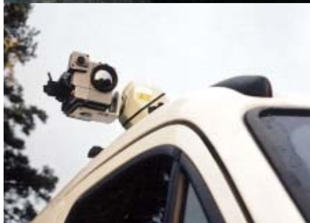
Arne Jensen AB has developed ever better techniques for checking district heating networks. Among other things, they have produced a solution in which the thermal camera is mounted on the roof of a vehicle and is controlled from a special panel inside the vehicle.
